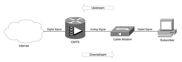
Conversely, the signals that pass to the CMTS from the provider network are considered downstream signals. The CMTS converts digital signals from the provider network into modulated analog signals that can be transmitted onto the coaxial cable line. The modulated analog signals are received by a CM at the subscriber site, where they are demodulated into a digital data stream suitable for transmission directly to the subscriber.
