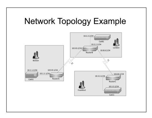
In the example network topology diagram above, the network is divided into three geographical areas: Boston, London, and Frankfurt. Each geographical area is represented by a gray rectangle. Boston's RouterA is connected to London's RouterB by using a T3 line. The two routers operate on the 10.9.9.0/24 network, wherein RouterA has been assigned an IP address of 10.9.9.1 and RouterB has been assigned an IP address of 10.9.9.2.
